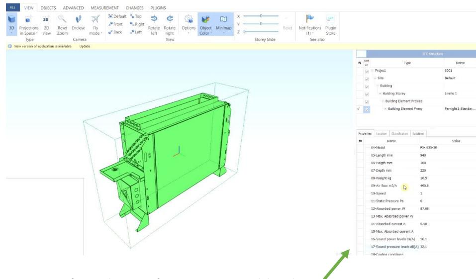
Parameters from Selection software are integrated directly in **Revit (or other BIM software)**
